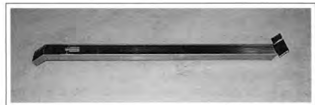
Figure 1-86. A simple kicker cut from 3\frac{5}{8} -inch stud. One shoe has been flattened out and beveled to fit flat to the surface it's fastened to.
