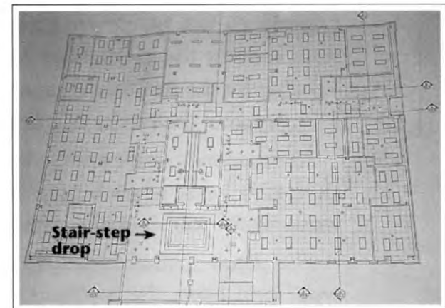
Figure 1-4. The reflective ceiling plan shown here breaks this floor of the building into “grid ceilings” and “hard lids.” You can also see a large stair-step drop in the entry way in the rectangle grid near the bottom of the plan. The lines around the rectangle show the separate widths of the stair-steps. The detail symbol cutting through the drop will give the rest of the information.
