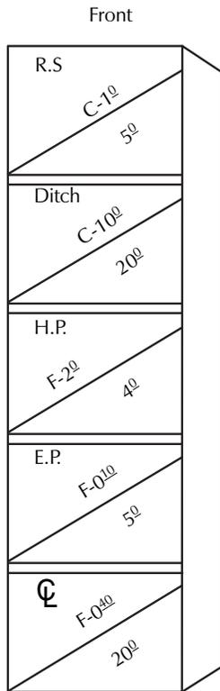
**Figure 1-2** Cut stake with double lines
