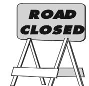
Type I, 2' wide, 3' high, Top panel 12" height, 1 reflectorized rail each side
